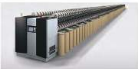
■ "BD" Open End Spinning Machine Saurer, Switzerland
